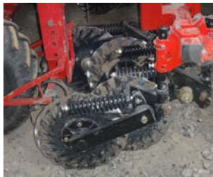
Combination rotating harrow synchrospire Franquet (backside tractor)
