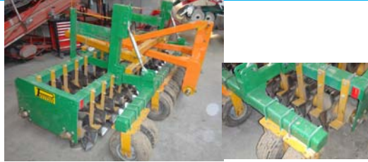
NivelSem + counterweight of 200 - 400 kg in front (in front of tractor)
